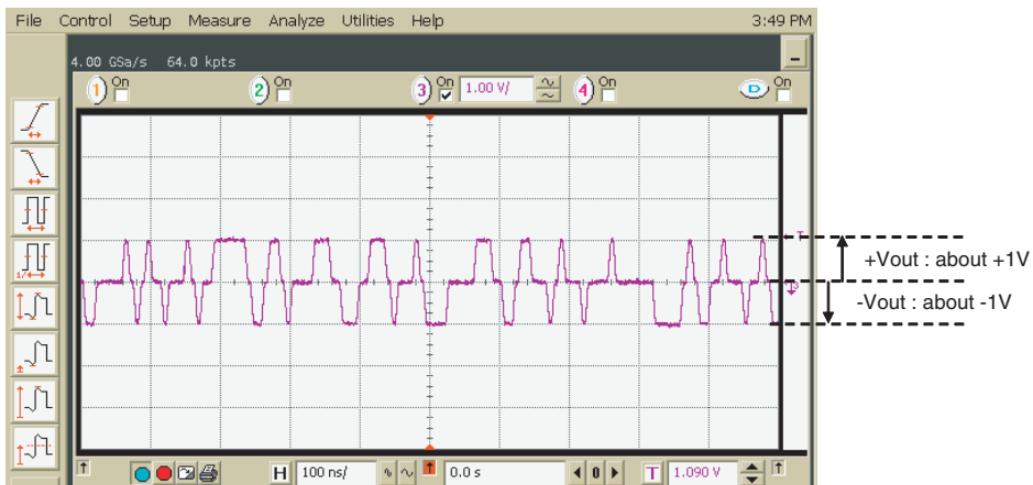
② 100Base-TX waveform 2 (A part of the waveform1 is magnified.)
